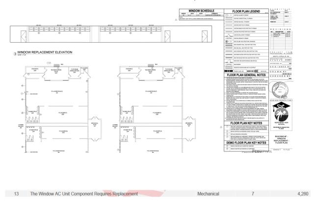
Per sheet A.100 Note 13 "Replace Window AC Component. Refer to Mech Dwgs". On Mech Drawings M.001 the wall package unit are included as part of the mechanical schedule.
